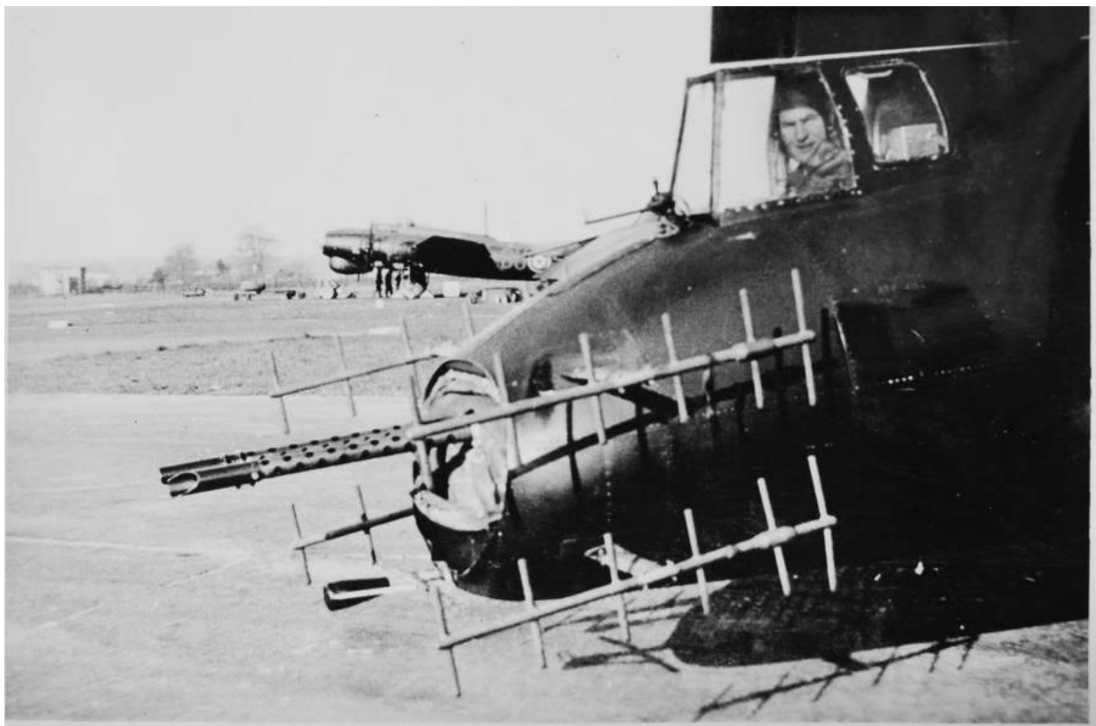
RNZAF Gunner L Budge in a 214 Squadron Fortress. Radar aerials are for the Airborne Grocer radar jamming equipment.
