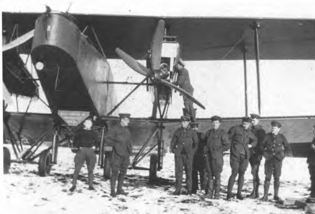
A change of propellers for O/100 3122 of 7A/14(N) Sqn. Beneath the nose is a landing light and, above it, is the bomb sight. :R.J. Neve
