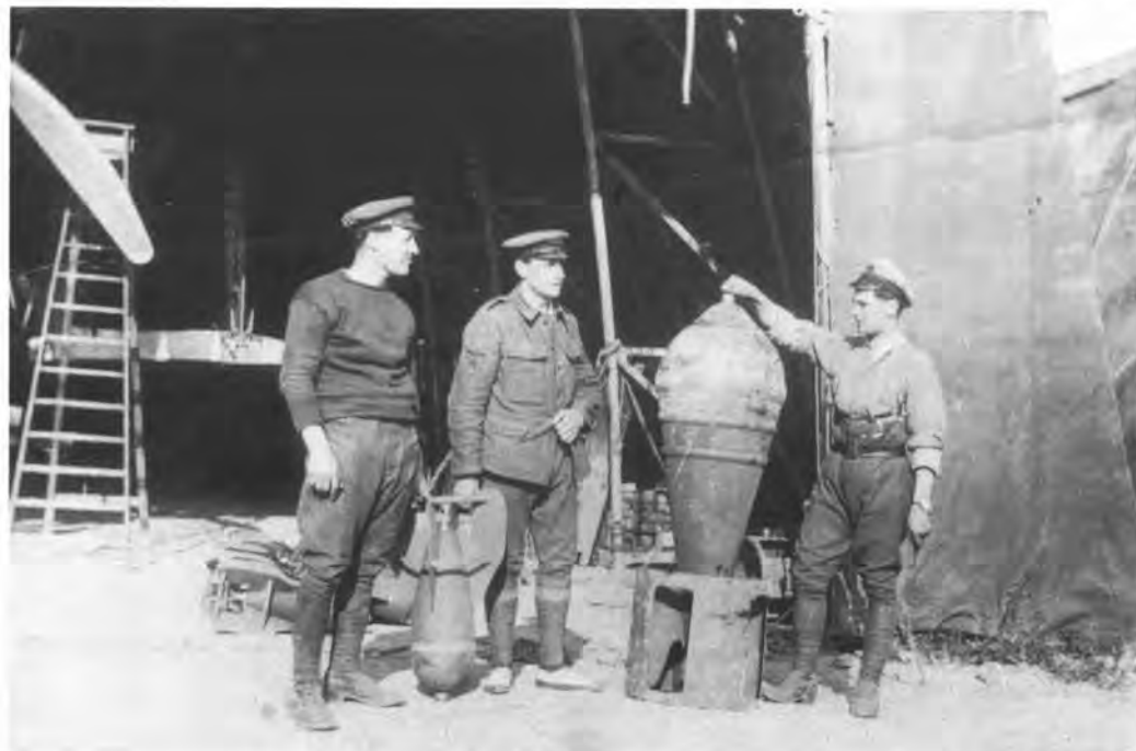
Coudekerque, 1917. Observer/Gunlayer Neve (on the right) illustrates the size of the 500lb HE bomb. On the left, its smaller brother is a 112lb HE bomb. Behind is a 'Nestler' portable hangar housing an 0/100 with its outer wings folded back. :R.J. Neve
