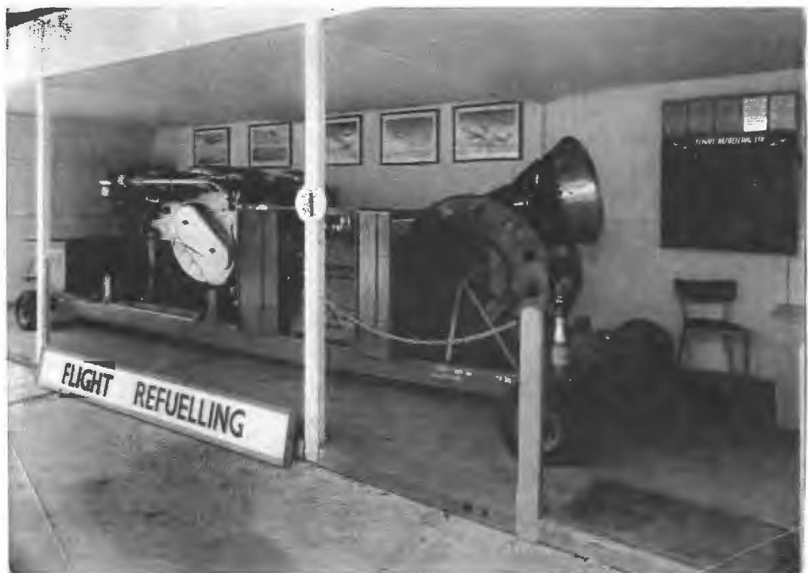
The Mark 16 Hose Drum Unit and Drogue
